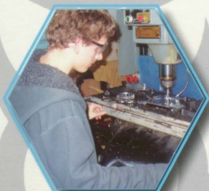
▲ John Saunders drills a piece of aluminum for the new robot.
